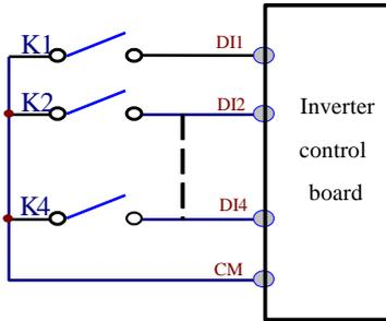
2. Wiring for active source electrode
