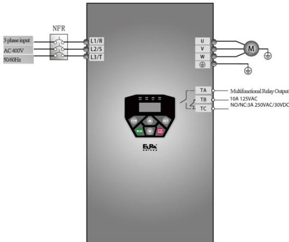
Figure 5-1 Wiring Diagram
