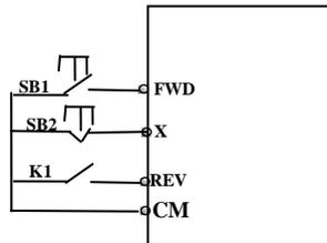
5. Start/stop controlled by direction pulse:
