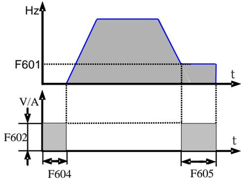
**Figure 5-18 DC braking**
