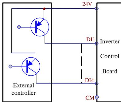
**Wiring by source electrode is a mode most in use at present. Wiring for control terminal is connected by source electrode, user should choose wiring mode according to requirement.**
