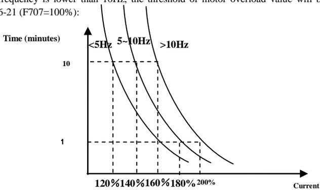
**Fig 6-21 Motor overload protection value**
