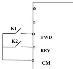
2. Two-line mode 2: when this mode is used, FWD is enable terminal, the direction is controlled by REV terminal.
