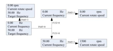
Fig 5-4 Operating flow chart of status parameter display
