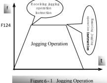
terminal (such as DI1) connected to CM, and inverter will run to jogging frequency. The rated function codes are from F316 to F323
