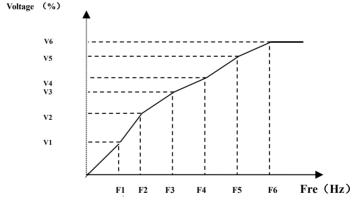
Fig 6-4 Polygonal-Line Type V/F
