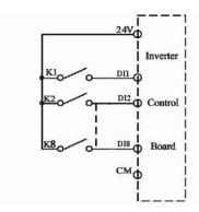
4. Wiring for active drain electrode (PNP mode)
