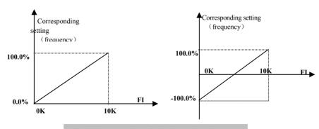
Fig 6-15 correspondence of pulse input and setting
