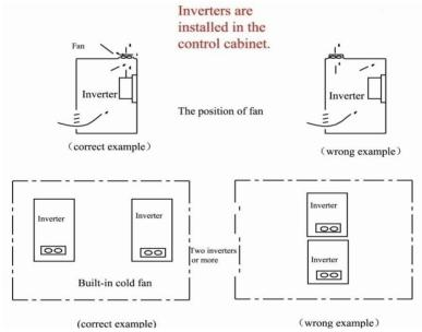
Fig 1-3 Installed in the cabinet
