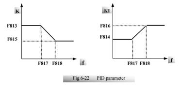
Dynamic response of vector control speed can be adjusted through adjusting proportional and storage gains of speed loop. Increasing KP and decreasing KI can speed up dynamic response of speed loop. However, if proportional gain or storage gain is too large, it may give rise to oscillation.
