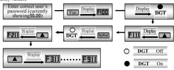
Fig 3-6 Switch over in a Code Group or between Different Code-Groups
