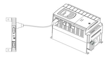
Fig 9-5 CANopen card installation
