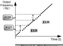
·Inverter will not skip this frequency span during acceleration/deceleration.
