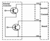
If digital input control terminals are connected by drain electrode, please turn the toggle switch to the end of "PNP". Wiring for control terminals as follows:
