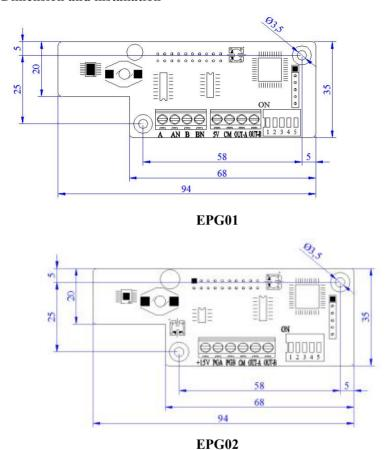
For 5.5KW and above 5.5kW inverters, the expansion card is installed inside of inverter. The card is installed nearby control board, which is fastened by 3\*5 self-tapping screw. J4 connector is connected to J10 in the control board by 20-core flat cable.
