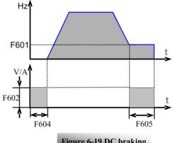
Figure 6-19 DC braking
