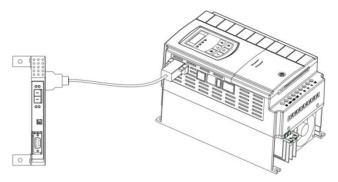
Fig 9-11 connection between communication card and inverter
