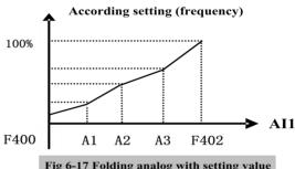
Fig 6-17 Folding analog with setting value
