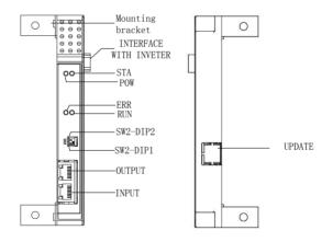
Fig 3 EtherCAT bus card
