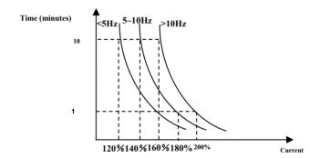
Fig 6-21 Motor overload protection value
