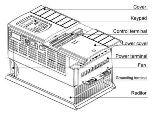
Metal housing uses advanced exterior plastic- spraying and powder-spraying process on the surface with elegant color and with detachable one-side door hinge structure adopted for front cover, convenient for wiring and maintenance. Taking E2000-0300T3 for instance, its appearance and structure are shown as in right Fig.
