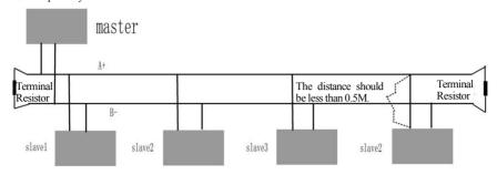
**Connecting Diagram of Terminal Resistance**
