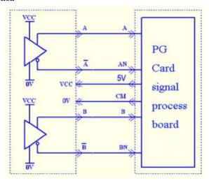
Differential output encoder (VCC=5V, please indicate it when differential encoder is selected).
