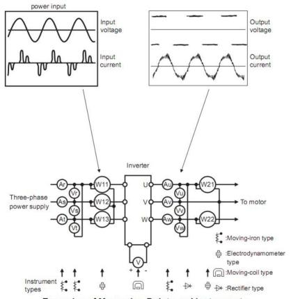
**Examples of Measuring Points and Instruments**
