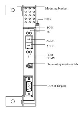
Fig 2-2 Communication card appearance and structure component
