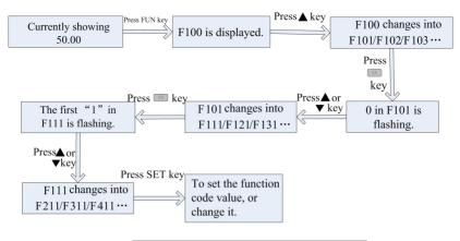
Fig 5-1 Switch over in a Code Group or between Different Code-Groups
