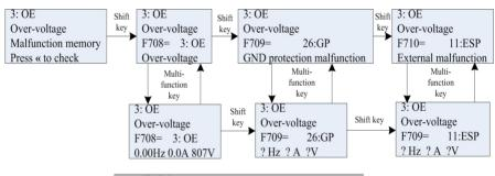
Fig 5-6 Operating flow chart of displayed malfunction interface
