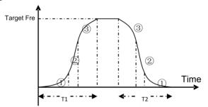
Fig 6-9 S curve acceleration /deceleration
